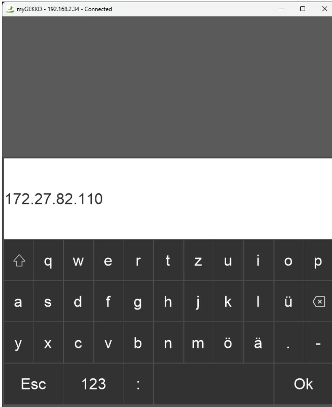
Once finished, please click on the "Ok" button to confirm it. You will be returned to the configuration menu. **NOTE:** if there is any mistake in the GW address, the IO-Station status will change to "Host address incorrect/Invalid certificate".
